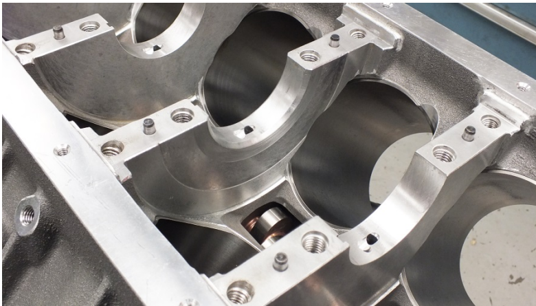
LS Next 2 Blocks come machined with clearance for fully counterweighted crankshafts
