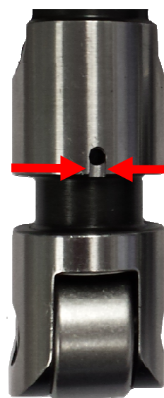
Figure 2: Dart oil galley modification from band to pushrod oil hole
