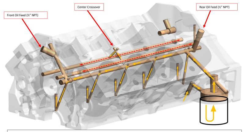
Oil flow comes in from the oil pump pickup, passes through the oil filter, up to the main oil galley, it is then diverted to the Main line (Crankshaft) bearings first (Priority main oiling) flows to the Cam bearings and then to the Lifter galleys secondary.
