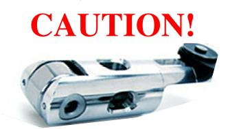
The use of lifters that are heavily lightened should not be used in Dart Blocks. The lightening holes will cause lifter oil to leak into the valley instead of oiling the pushrod, rocker arm and valvespring.
