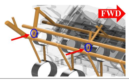
Oil Restrictor provisions are in-between the main oil feed and the Drivers side Lifter galley located in the center and rear crossovers in the valley. These are drilled and tapped for 1/8" NPT.
