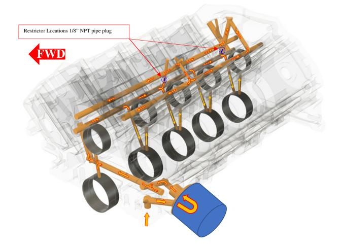
Oil flow comes in from the oil pump pickup, passes through the oil filter, up to the main oil galley feeding the #1 main and cam bearing on the way, it is then diverted to the Main line (Crankshaft) bearings first (Priority main oiling) flows to the Cam bearings and then to the Lifter galleys secondary.
